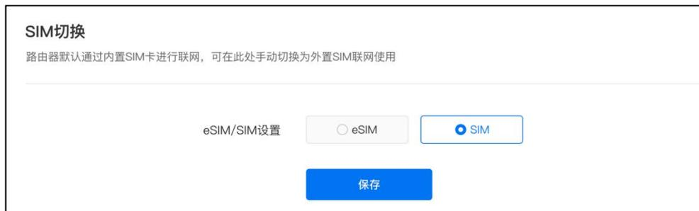
The screenshot shows the 'SIM切换' (SIM Switching) configuration page. At the top, it states: '路由器默认通过内置SIM卡进行联网，可在此处手动切换为外置SIM联网使用'. Below this, there is a section labeled 'eSIM/SIM设置' with two radio buttons: 'eSIM' (unselected) and 'SIM' (selected). A blue '保存' (Save) button is located at the bottom of the configuration area.
