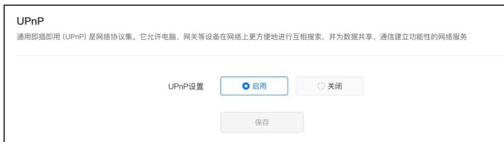
The screenshot shows the 'UPnP' configuration page. It includes a description: '通用即插即用 (UPnP) 是网络协议集。它允许电脑、网关等设备在网络上更方便地进行互相搜索，并为数据共享、通信建立功能性的网络服务'. The 'UPnP设置' (UPnP Settings) section has two radio buttons: '启用' (Enabled, selected) and '关闭' (Disabled). A grey '保存' (Save) button is positioned below the radio buttons.
